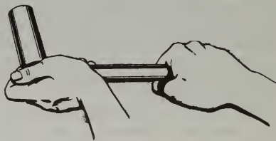
FIGURE 4-57. Proper spark plug removal technique.
